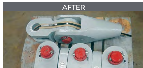
Mining wire rope attachments refurbished and recertified
